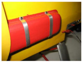
There is a large oil tank on the Moth so I carved one from balsa, stuck it on a ply backing plate and added litho plate straps. There's all sorts of junk under the fuel tank including fuel pipe, tap and assorted controls. I contented myself with
